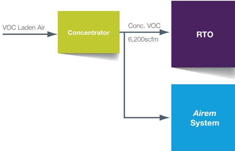
**Option C:** Flow VOC to Airem system and exhaust directly to RTO
